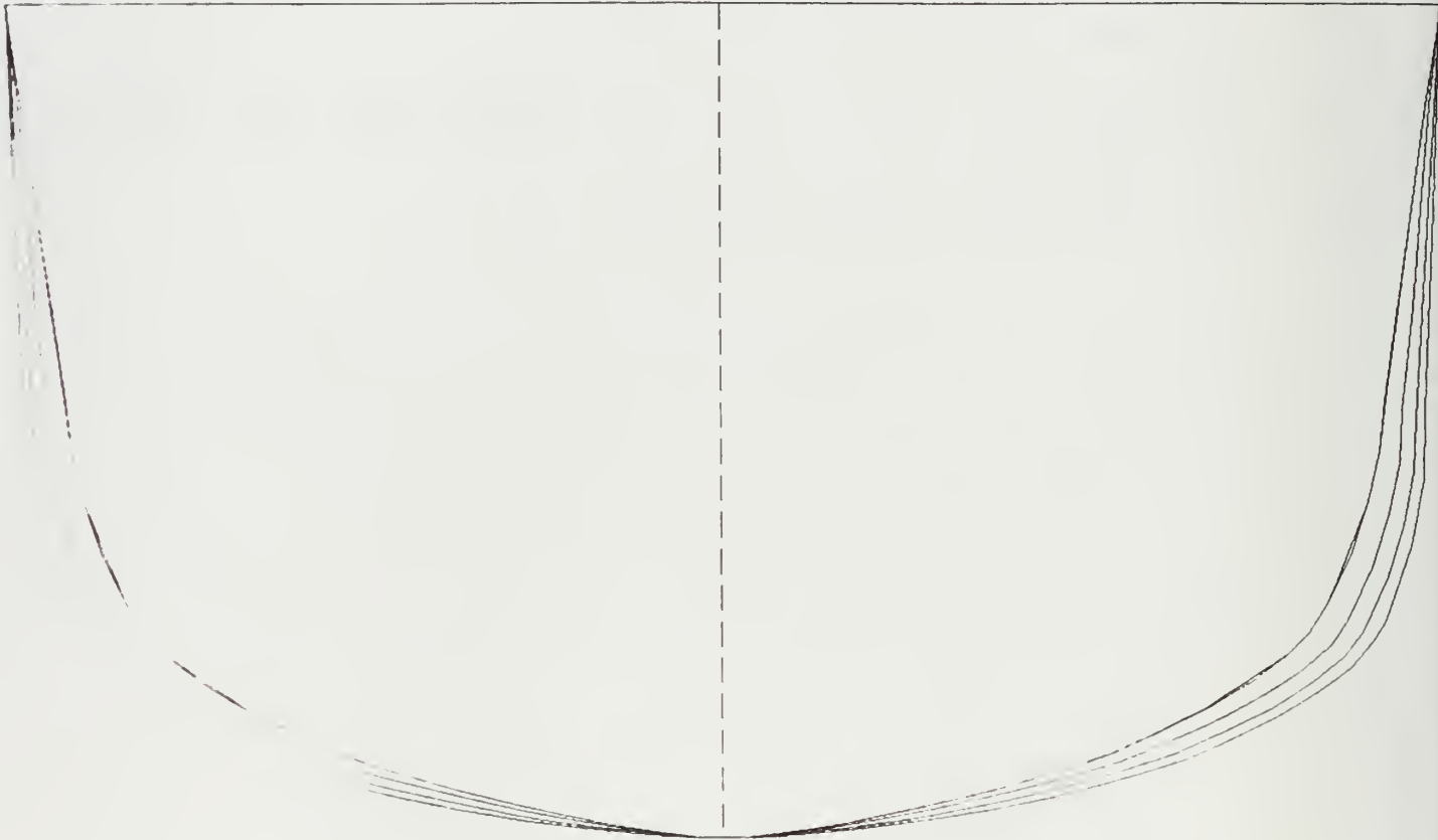
COMP_DA.C Body Plan (1 component) Scale = 1:100
